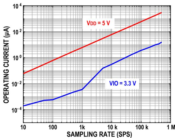
Figure 35. Operating Current vs. Sampling Rate
