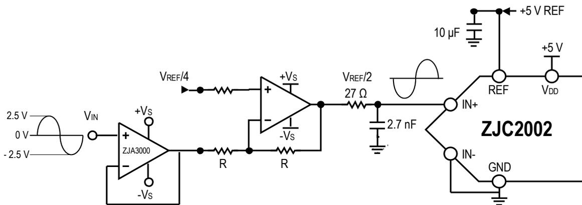
Figure 32. Single-ended Bipolar to Pseudo Differential Unipolar
