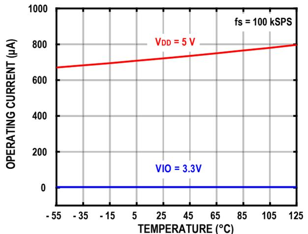
Figure 24. Operating Current vs. Temperature
