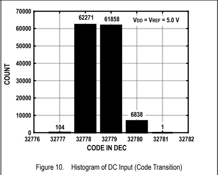
Figure 10. Histogram of DC Input (Code Transition)
