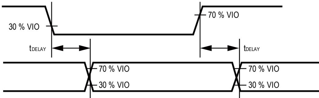
Figure 6. Voltage Levels for Timing
