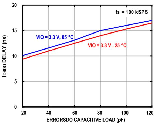
Figure 23. t<sub>psdo</sub> Delay vs Capacity Load and Voltage
