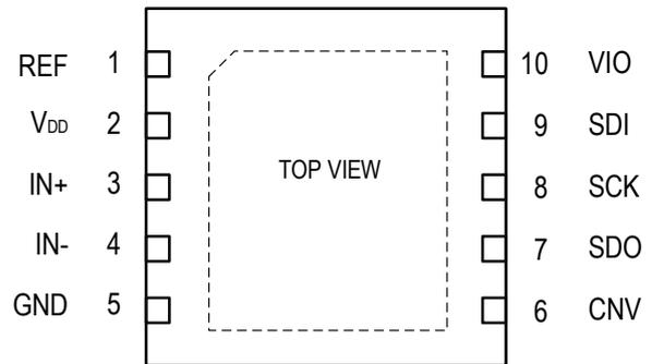
Figure 4. 10-lead DFN pin configuration
