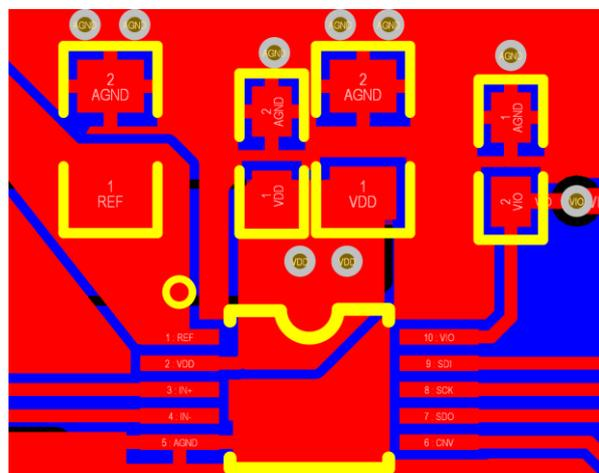
Figure 48. Example Layout and Routing of ZJC2002
