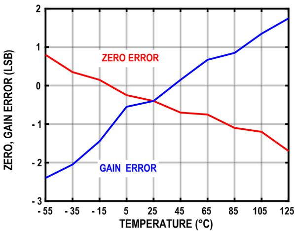
Figure 21. Zero Input, Gain Error vs. Temperature
