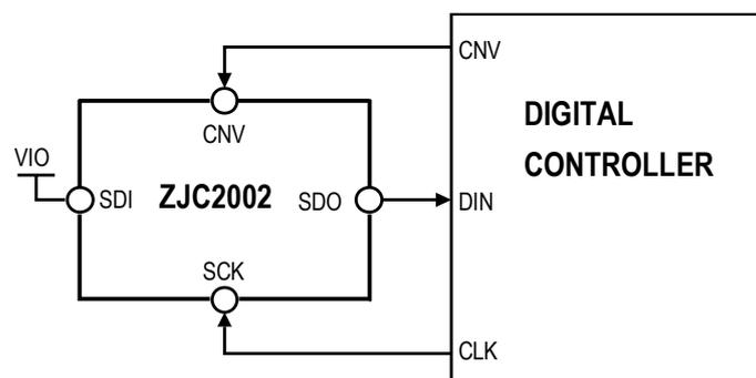
Figure 36.  $\overline{\text{CS}}$  Mode (3-wire without Busy Indication) Connection Diagram
