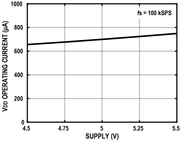
Figure 19. V<sub>DD</sub> Operating Current vs. Power Supply Voltage
