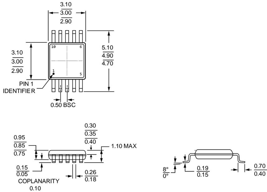
Figure 49. 10-Lead MSOP Package Dimensions Shown in Millimeter
