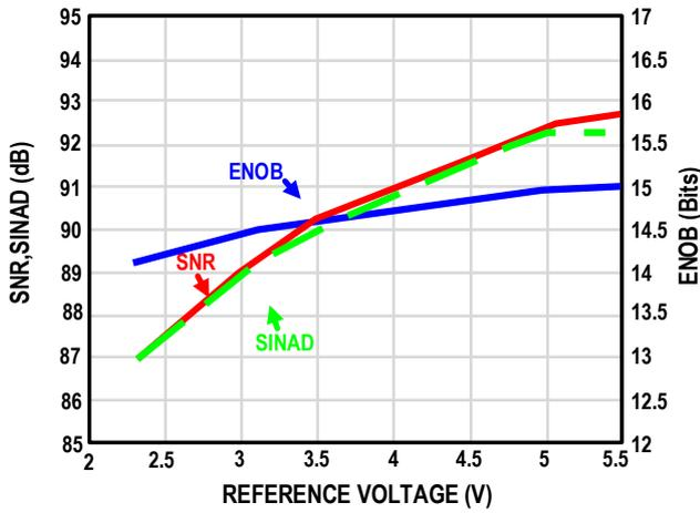
Figure 13. SINAD and ENOB vs. Reference Voltage
