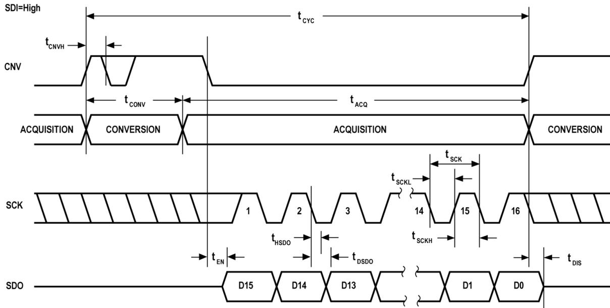
Figure 37.  $\overline{CS}$  Mode (3-Wire without Busy Indication) Serial Interface Timing
