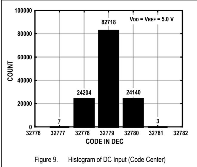
Figure 9. Histogram of DC Input (Code Center)
