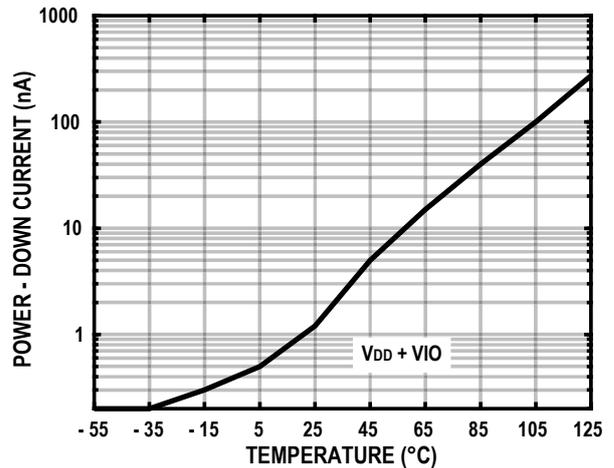
Figure 22. Stand-by Current vs. Temperature
