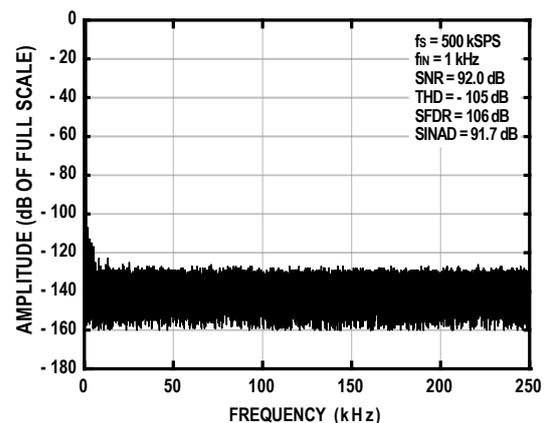
Figure 2. AC Characteristics
