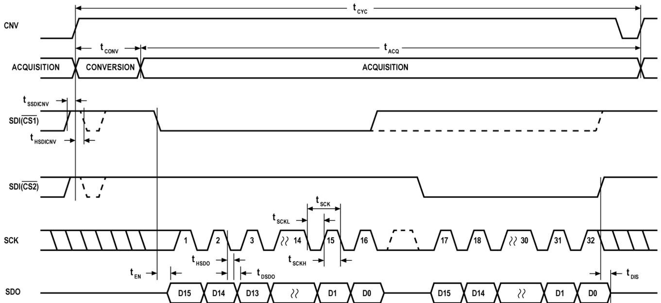
Figure 41.  $\overline{CS}$  Mode (4-Wire without Busy Indication) Serial Interface Timing
