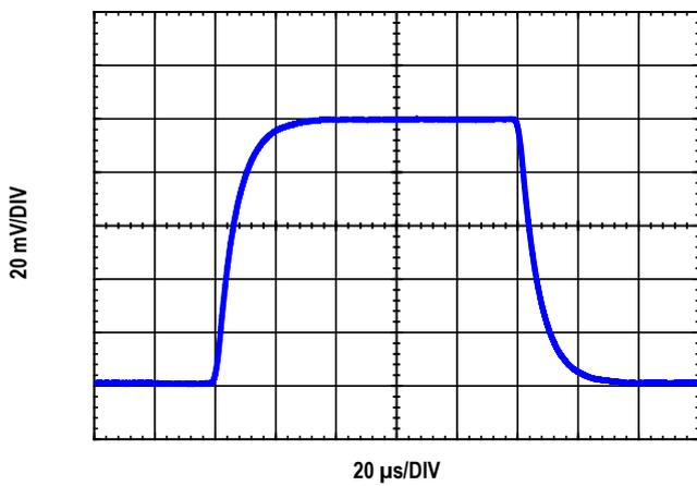
图24. 小信号响应 (G = 1000,  $R_L = 2\text{ k}\Omega$ ,  $C_L = 100\text{ pF}$ )
