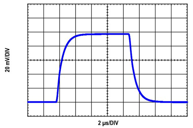
图23. 小信号响应 (G = 100,  $R_L = 2\text{ k}\Omega$ ,  $C_L = 100\text{ pF}$ )
