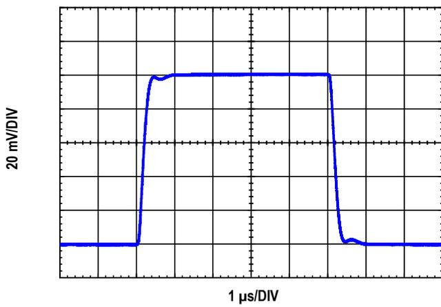
图22. 小信号响应 (G = 10,  $R_L = 2\text{ k}\Omega$ ,  $C_L = 100\text{ pF}$ )
