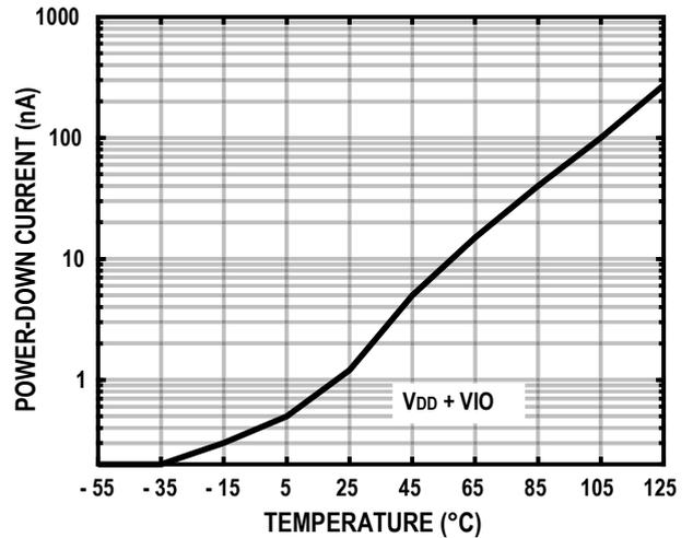
Figure 22. Stand-by Current vs. Temperature
