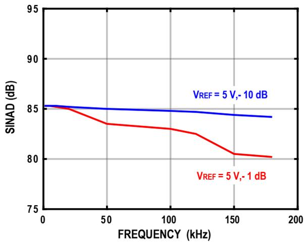
Figure 17. SINAD vs. Frequency
