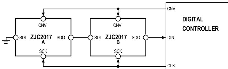
Figure 44. Chain Mode (without Busy Indication) Connection Diagram
