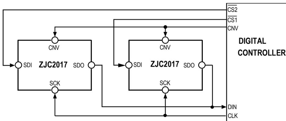
Figure 40.  $\overline{CS}$  Mode (4-wire without Busy Indication) Connection Diagram
