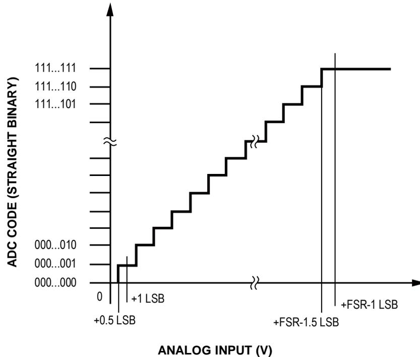
Figure 26. ADC Ideal Transfer Function
