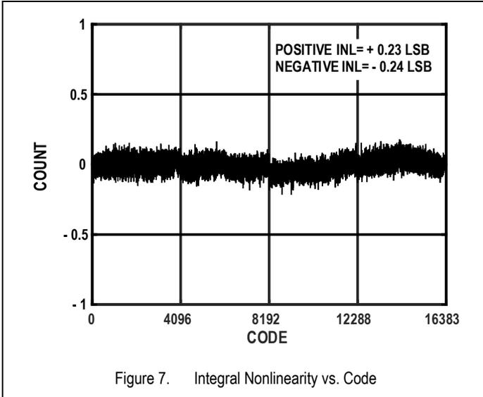
Figure 7. Integral Nonlinearity vs. Code
