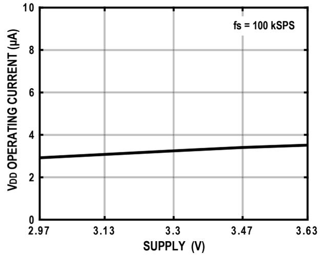
Figure 20. V<sub>IO</sub> Operating Current vs. Power Supply Voltage
