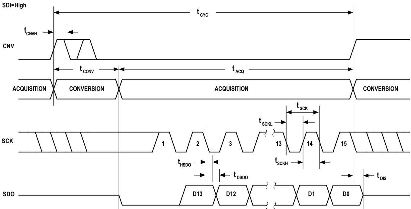
Figure 39.  $\overline{CS}$  Mode (3-Wire with Busy Indication) Serial Interface Timing
