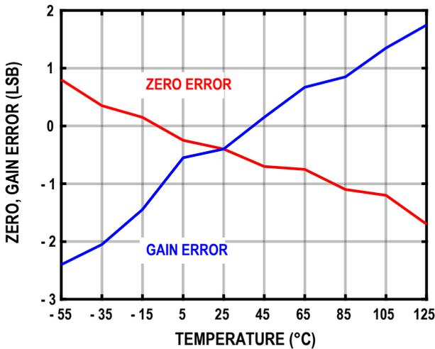
Figure 21. Zero Input, Gain Error vs. Temperature
