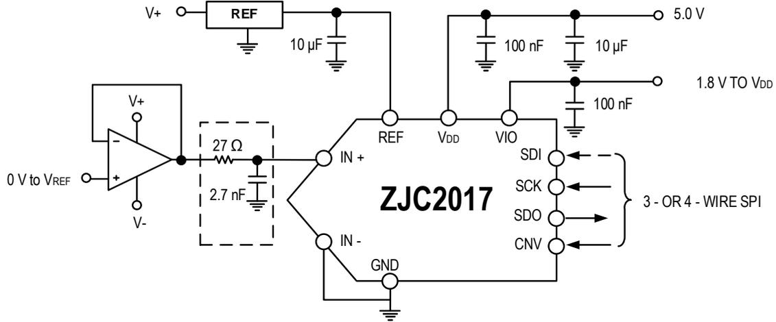
Figure 27. Application Circuits Using Multiple Power Supplies
