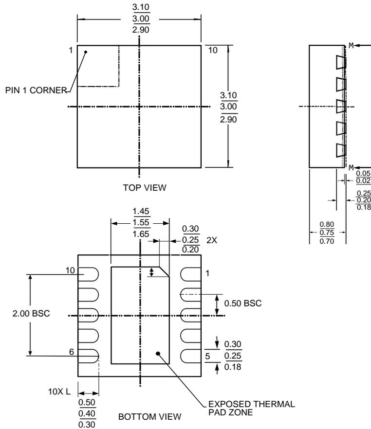
Figure 50. 10-Lead DFN Package Dimensions Shown in Millimeter
