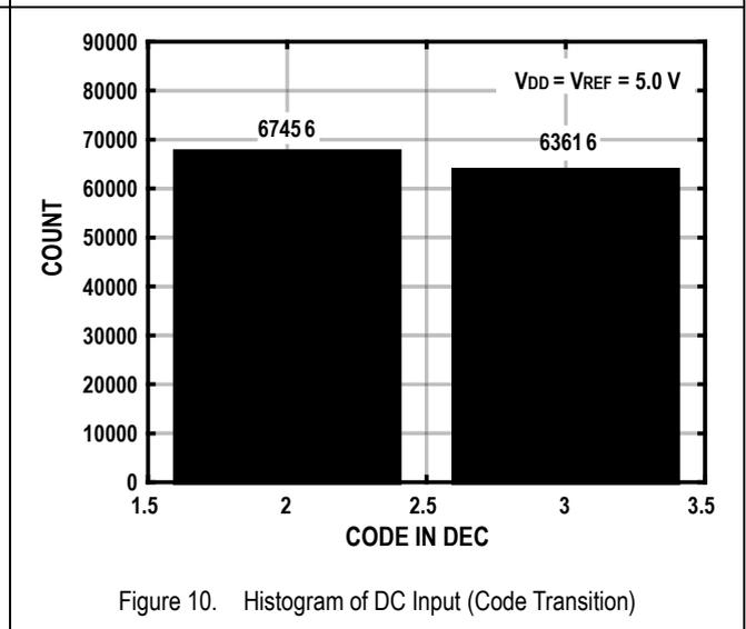
Figure 10. Histogram of DC Input (Code Transition)
