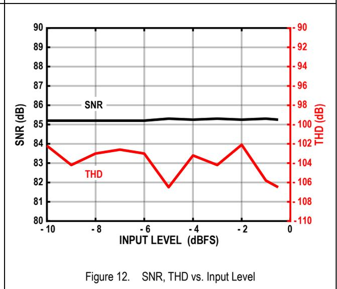
Figure 12. SNR, THD vs. Input Level
