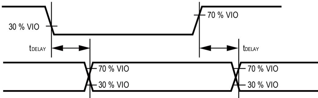
Figure 6. Voltage Levels for Timing
