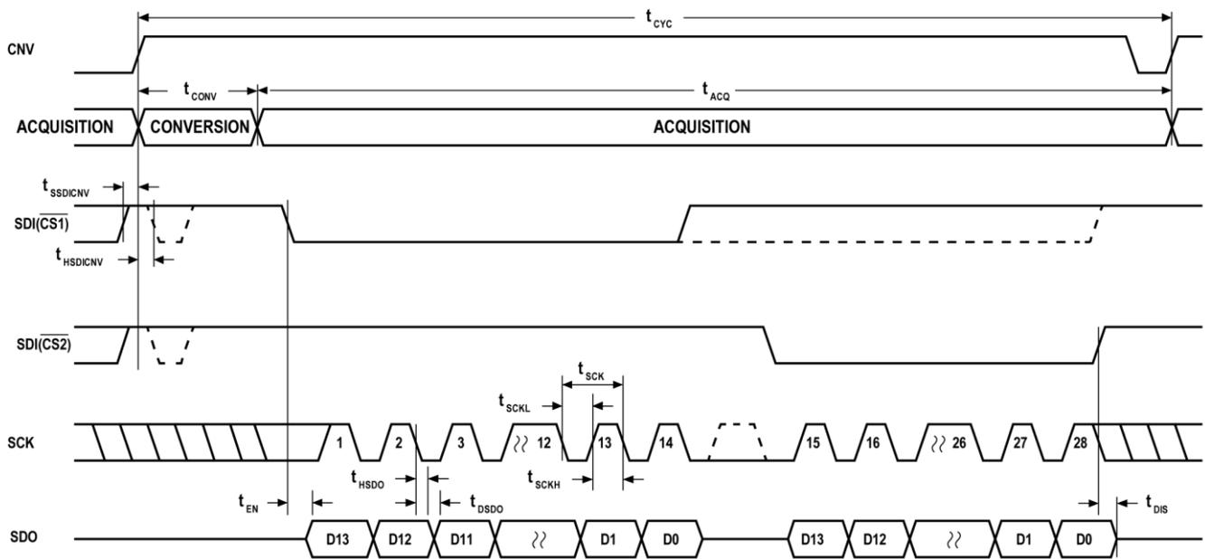
Figure 41.  $\overline{CS}$  Mode (4-Wire without Busy Indication) Serial Interface Timing
