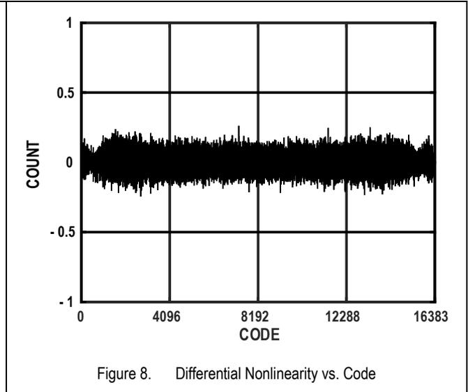
Figure 8. Differential Nonlinearity vs. Code
