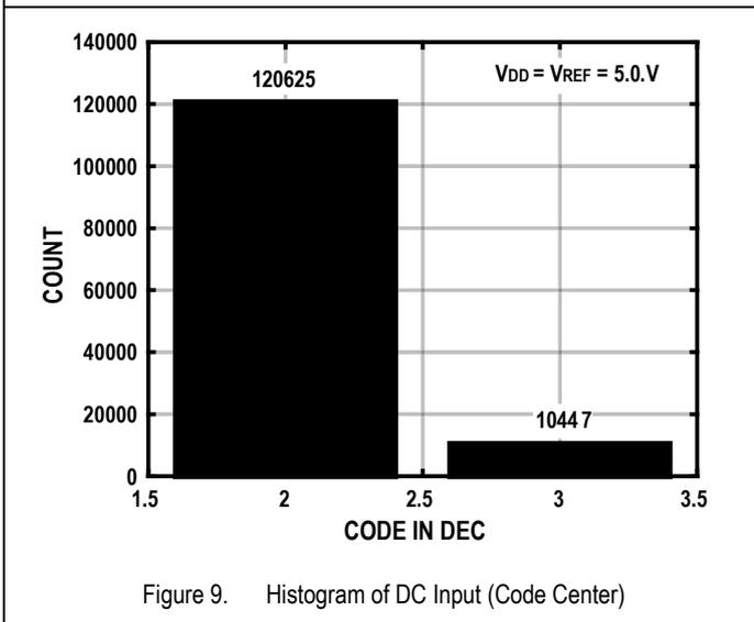
Figure 9. Histogram of DC Input (Code Center)
