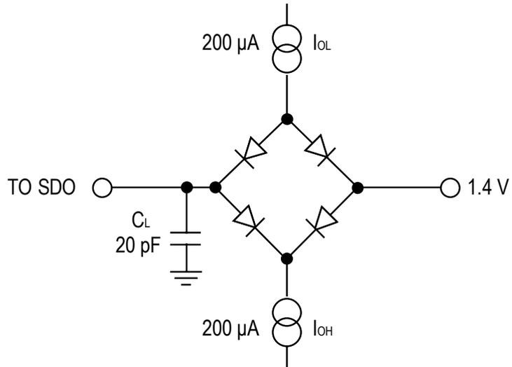
Figure 5. Load Circuit for Digital Interface Timing
