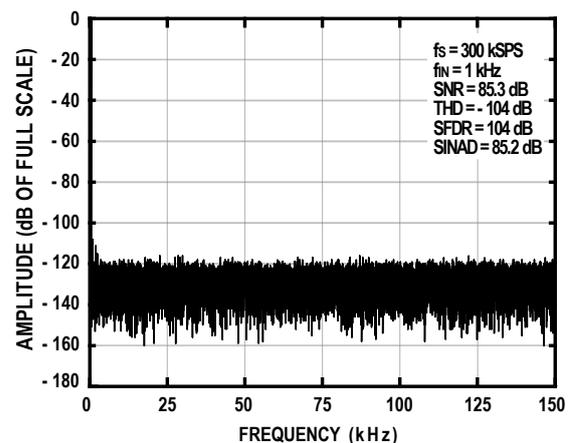
Figure 2. AC Characteristics
