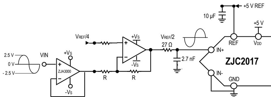
Figure 32. Single-ended Bipolar to Pseudo Differential Unipolar
