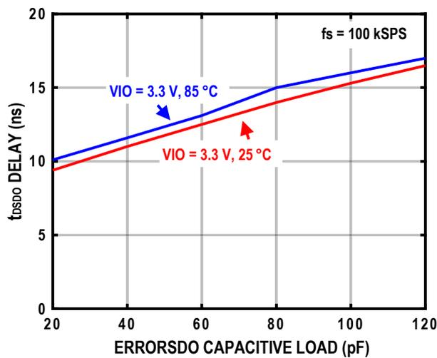
Figure 23. t<sub>SDO</sub> Delay vs. Capacity Load and Voltage
