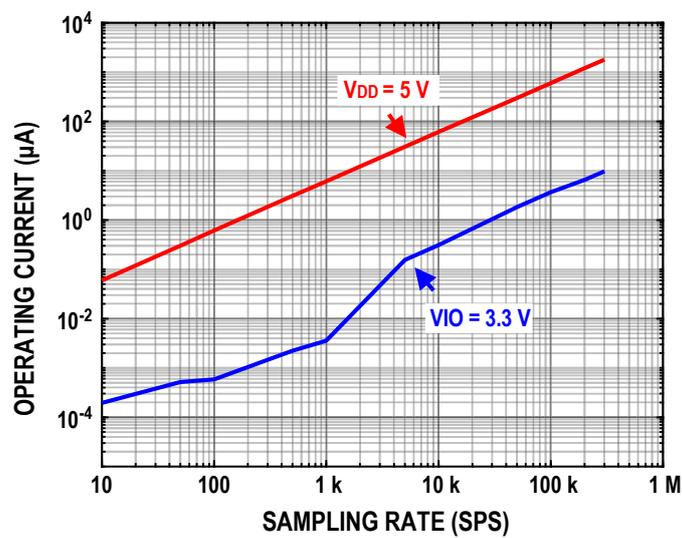
Figure 35. Operating Current vs. Sampling Rate
