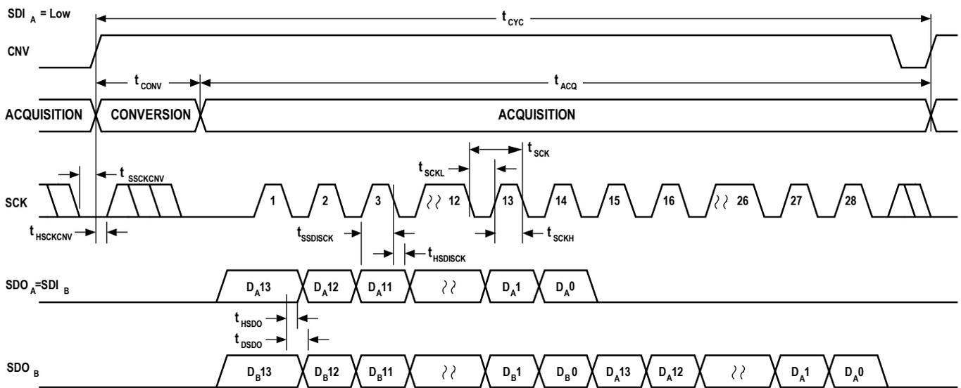
Figure 45. Chain Mode (without Busy Indication) Serial Interface Timing
