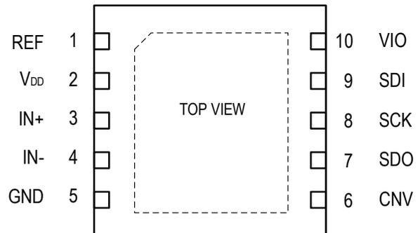
Figure 4. 10-lead DFN Pin Configuration
