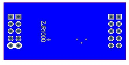
Figure 28. ZJR1000 Evaluation Board Layout (Bottom Layer)
