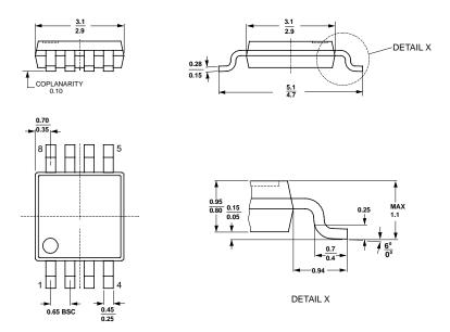
Figure 30. 8-Lead MSOP Package Dimensions shown in millimeters
