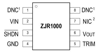
Note: 1 DNC = Do Not Connect; 2 NIC = No Internal Connection Figure 1. ZJR1000 Pin Configuration (8-lead SOIC and MSOP)
