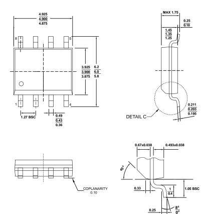
Figure 29. 8-Lead SOIC Package Dimensions shown in millimeters
