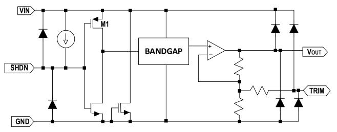
Figure 20. Simplified Schematic of ZJR1000
