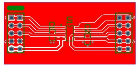
Figure 27. ZJR1000 Evaluation Board Layout (Top Layer)
