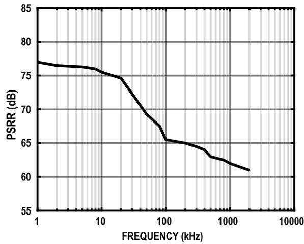
Figure 36. PSRR vs. Frequency
