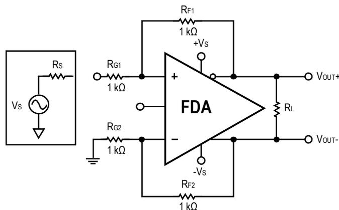
Figure 33. Realizing Bipolar Single-Ended to Fully Differential via Differential Op Amp
