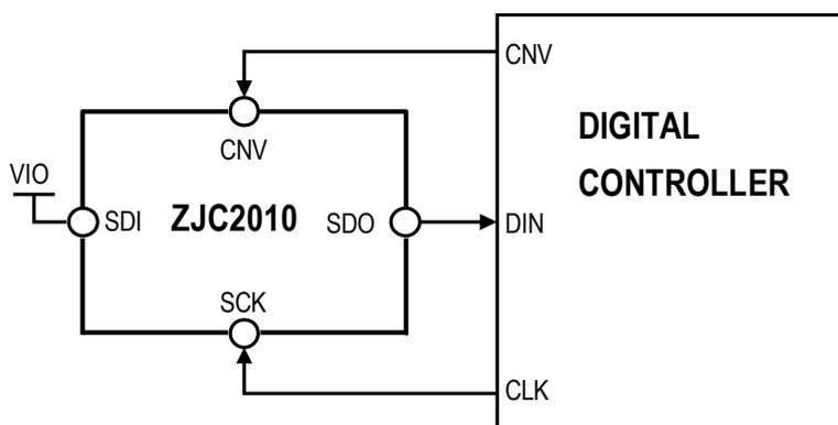
Figure 38.  $\overline{\text{CS}}$  Mode (3-wire without Busy Indication) Connection Diagram
