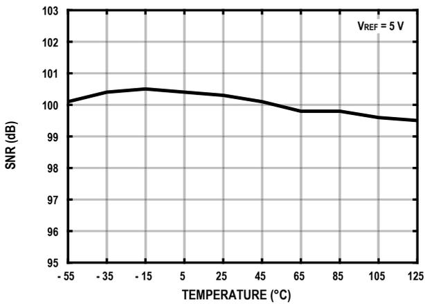
Figure 15. SNR vs. Temperature
