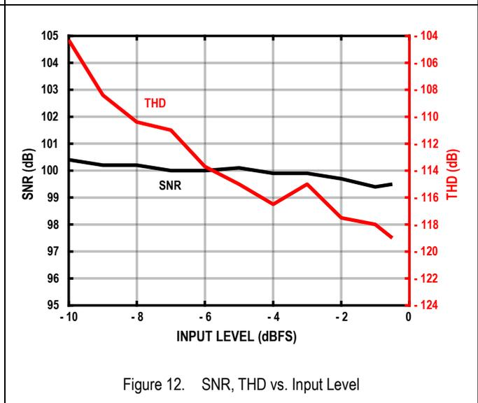
Figure 12. SNR, THD vs. Input Level
