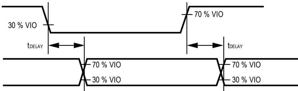
Figure 6. Voltage Levels for Timing
