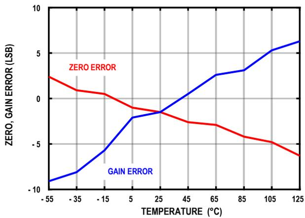
Figure 21. Zero Input, Gain Error vs. Temperature
