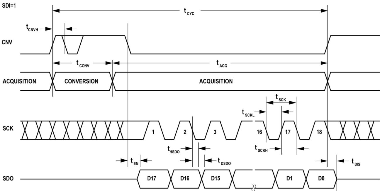
Figure 39.  $\overline{CS}$  Mode (3-Wire without Busy Indication) Serial Interface Timing
