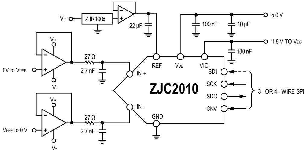
Figure 27. Application Circuits Using Multiple Power Supplies
