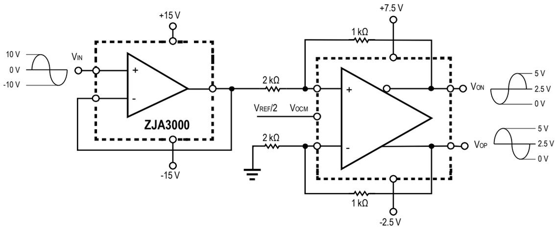
Figure 34. High Input Impedance Bipolar Single-ended to Fully Differential
