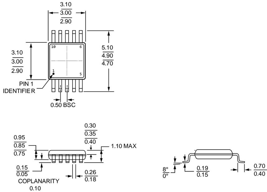
Figure 51. 10-Lead MSOP Package Dimensions Shown in Millimeter
