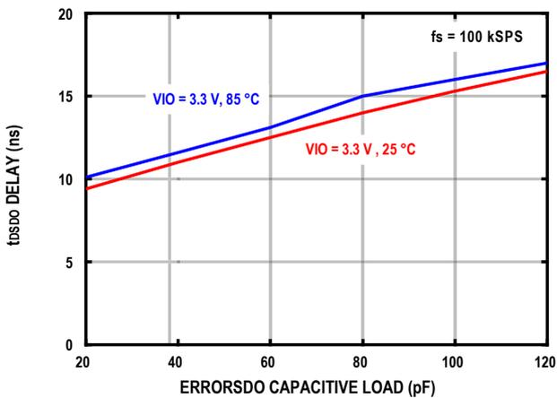
Figure 23.  $t_{BSDO}$  Delay vs. Capacity Load and Voltage
