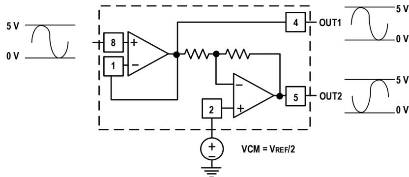
Figure 32. High Input Impedance Unipolar Single-Ended to Fully Differential
