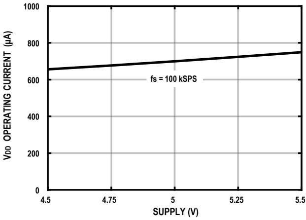
Figure 19.  $V_{DD}$  Operating Current vs. Power Supply Voltage
