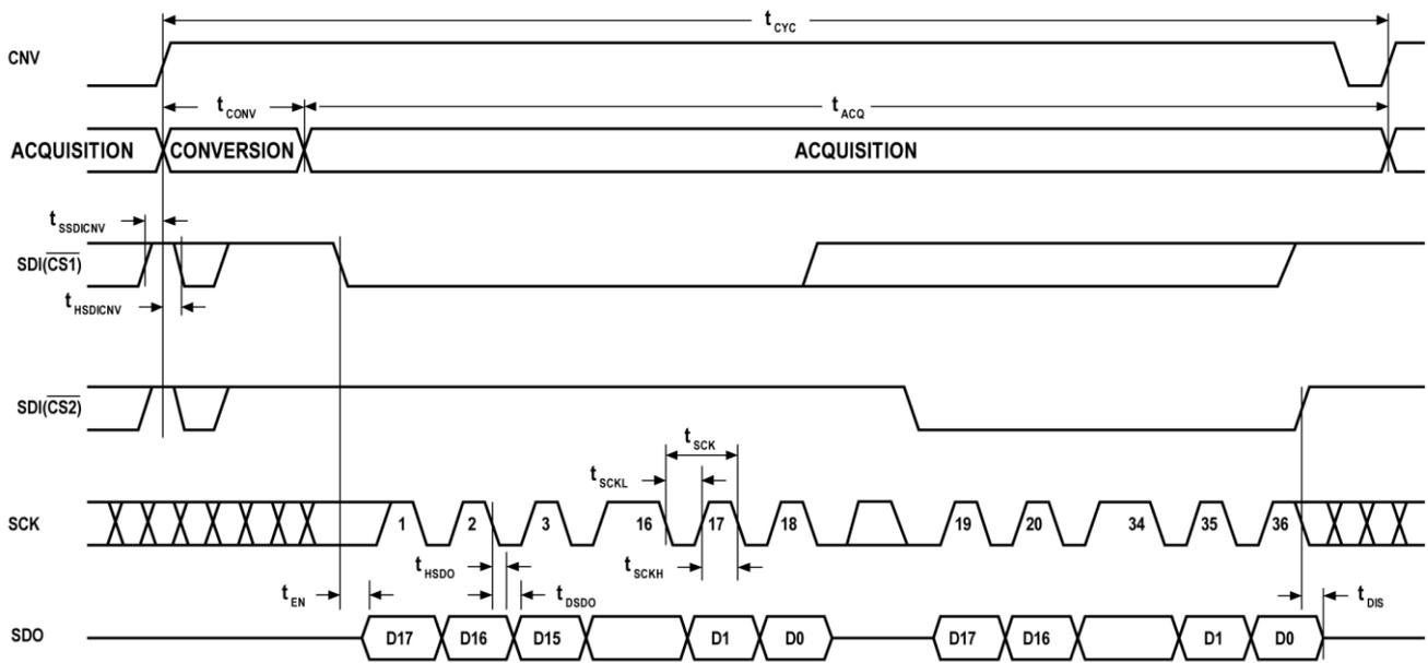
Figure 43.  $\overline{CS}$  Mode (4-Wire without Busy Indication) Serial Interface Timing
