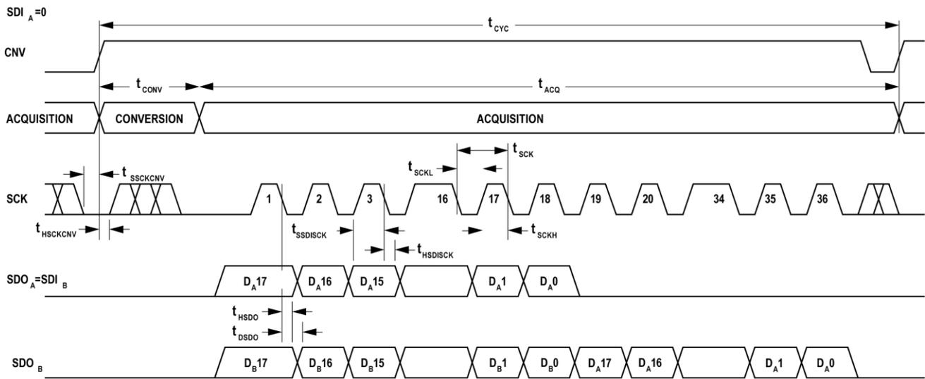
Figure 47. Chain Mode (without Busy Indication) Serial Interface Timing
