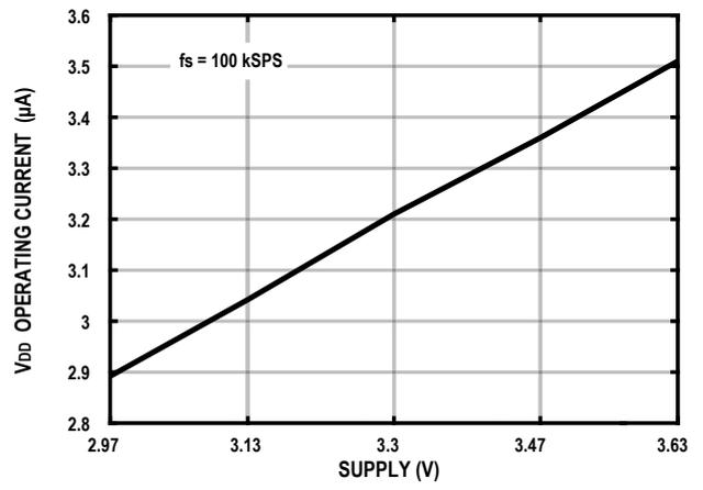
Figure 20.  $V_{IO}$  Operating Current vs. Power Supply Voltage
