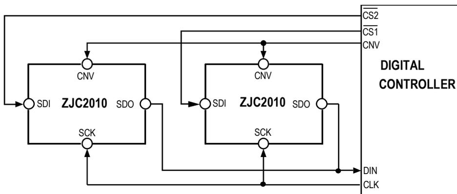
Figure 42.  $\overline{CS}$  Mode (4-wire without Busy Indication) Connection Diagram
