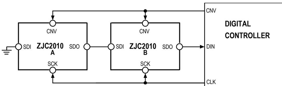
Figure 46. Chain Mode (without Busy Indication) Connection Diagram
